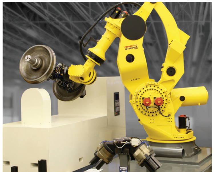
M-2000iA/1200 heavy payload machining
